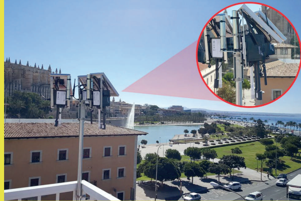
Figure 2. IoT environmental sensor installed in the Port Authority of Palma's headquarters
